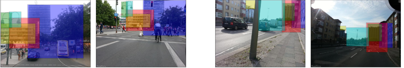
Fig. 1: We present a novel place recognition system that adapts state-of-the-art object proposal techniques to identify potential landmarks within an image. The proposed system utilizes convolutional network features as robust landmark descriptors to recognize places despite severe viewpoint and condition changes, without requiring any environment-specific training. The colored boxes in the images above show ConvNet landmarks that have been correctly matched between two significantly different viewpoints of a scene, thus enabling place recognition under these challenging conditions.
