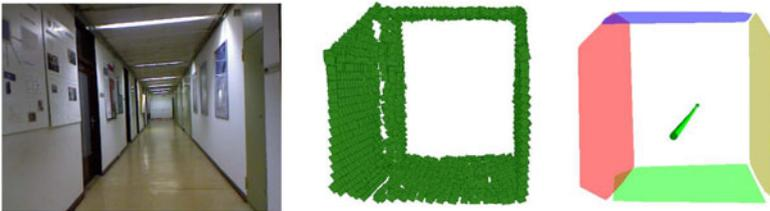
**Fig. 5** (left) RGB image of the corridor. (mid) Downsampled point cloud containing about 3,000 points. (right) Extracted planes of the walls. The planes have been classified into floor, ceiling, left, and right wall. The green arrow shows the intended motion direction computed from the position and orientation relative to the walls.
