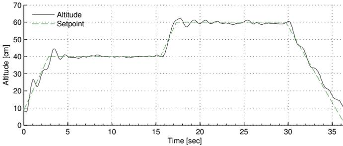
**Fig. 4** Altitude plot showing a take-off, altitude-hold at 40 cm followed by an altitude-hold at 60 cm and a landing maneuver. The altitude setpoint is automatically increased and decreased in a ramp. Note that the sonar sensor is mounted about 10 cm above ground.
