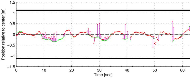
**Fig. 6** Position estimates of the quadrotor within the corridor during autonomous flight, based on the Kinect measurements. The red points represent the calculated distances based on the left wall and the green points are based on the right wall. If two walls are visible, measurements are connected through a line. The corridor walls are shown as thick black horizontal lines. The maximum deviation from the corridor center was 35 cm.
