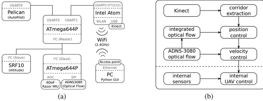
**Fig. 3** (a) Schematic diagram of the main components and their communication channels. (b) Cascaded controller structure and main sensors used. For reasons of clarity the altitude controller is not shown here. It operates parallel to the position and velocity controller and uses an SRF-10 sonar sensor to measure the altitude.
