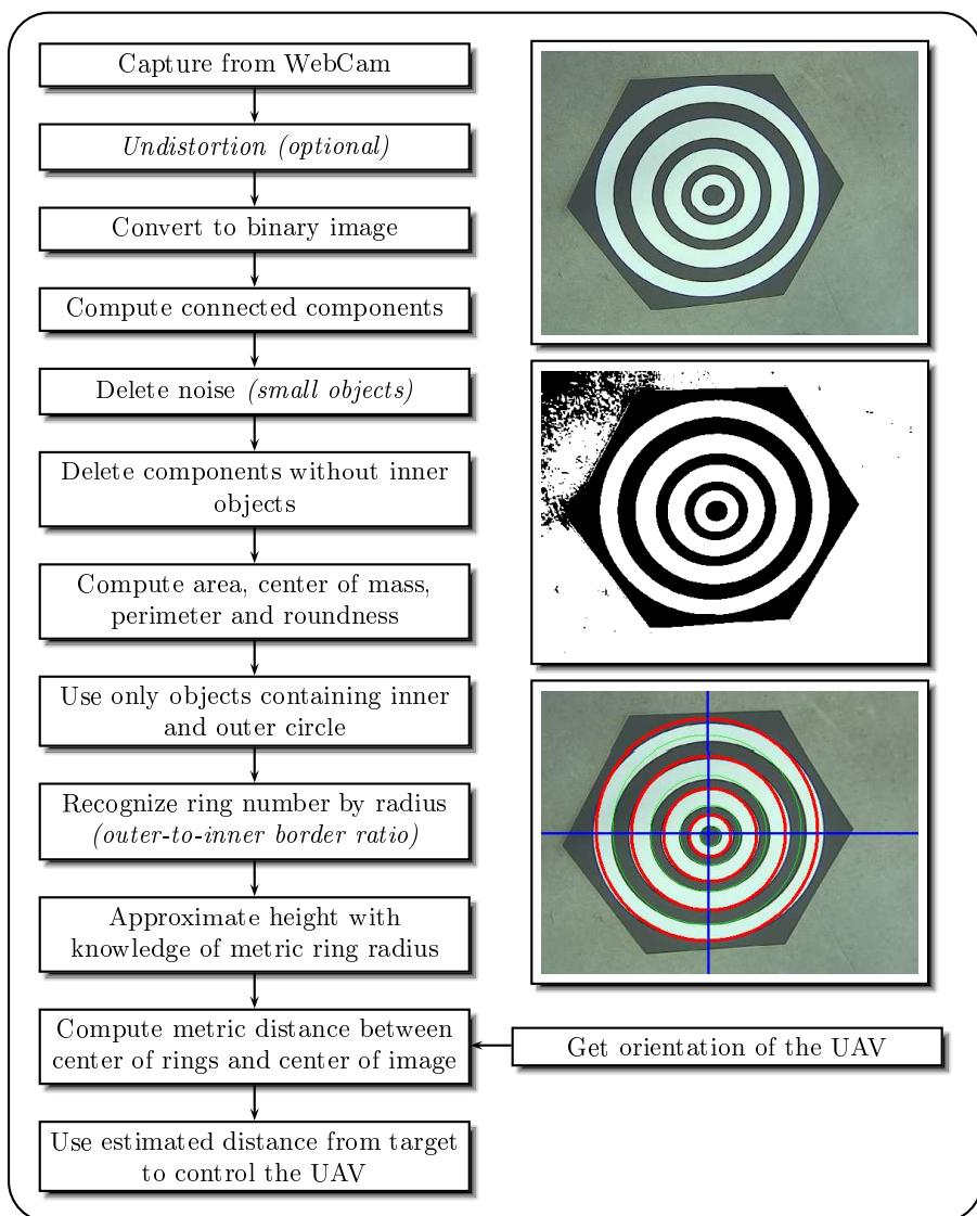
**Fig. 2.** Algorithm for landing pad detection
