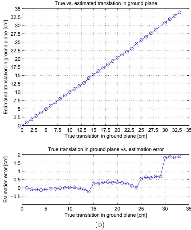
**Fig. 5.** True vs. estimated translation in ground plane and corresponding errors
