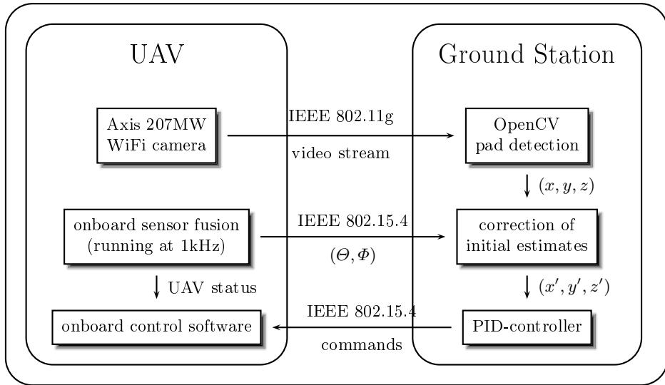
**Fig. 3.** System architecture and flow of information
